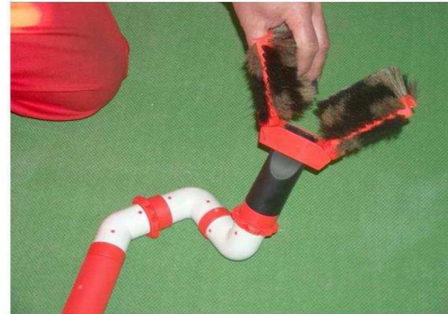
Fig. 9: Forked brush (H091-08) with special 2x90° swivel elbow (H091-05S) and 135° elbow (H091-06) for rotating the brush around the insulator
