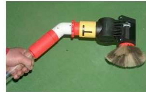
Fig. 10: Turbo brush (H091-14) with 135° elbow (H091-06) for cleaning petticoat insulators
