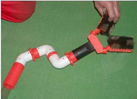
Fig. 9: Forked brush (H091-08) with special 2x90° swivel elbow (H091-05S) and 135° elbow (H091-06) for rotating the brush around the insulator
