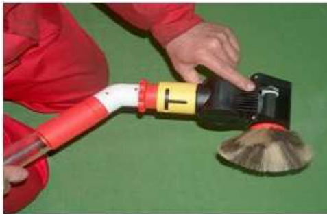
Fig. 10: Turbo brush (H091-14) with 135° elbow (H091-06) for cleaning petticoat insulators
