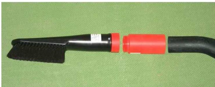
Fig. 15: Using the conical connector for attaching cleaning components directly to the vacuum cleaner hose (for cleaning equipment for live working up to 1 kV).
