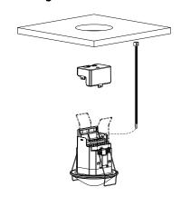
Installation in false ceilings for ceiling thicknesses of 0.5mm to 3cm. The diameter of the ceiling cutout must be between 62mm and 70mm. The cable strain relief is implemented using a cable tie (width: 3.5-4.8mm).
