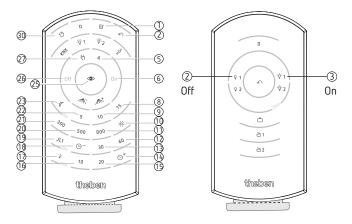
① If the command sent from the presence detector is accepted, the red LED flashes briefly twice. If the command is rejected, the red LED flashes briefly once.
