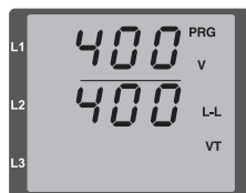
Fig. Voltage transformer programming mode Buttons 1 and 2 can be used to modify the primary and secondary voltage (cf. page 52).
