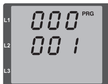
Fig. Parameter screen programming mode Buttons 1 and 2 can be used to modify the individual parameters (cf. page 47).
