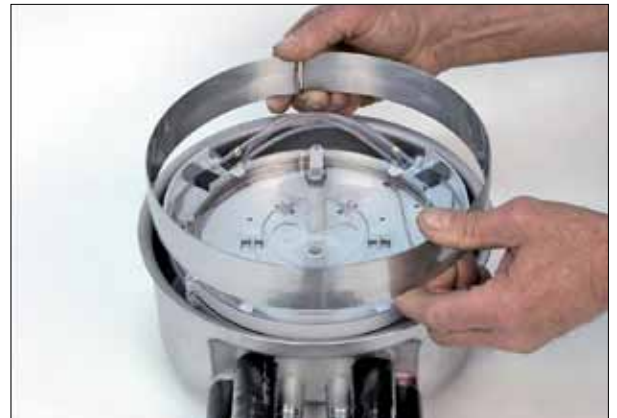
Mounting of support sleeve
