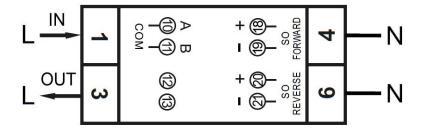
When connecting the meter through a serial converter (RS485) for testing, please be aware that because of not implementing the complete Modbus infrastructure, there will be a need to put an additional resistor (120 ohms/ 0.25 watts) across the terminals (10 & 11) on the meter side.
