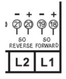
pin 18/20 (collector) pin 19/21 (emitter)
