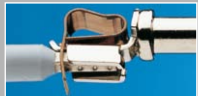
fine-wire - with wire-end ferrule, gas-tight, crimped-on
