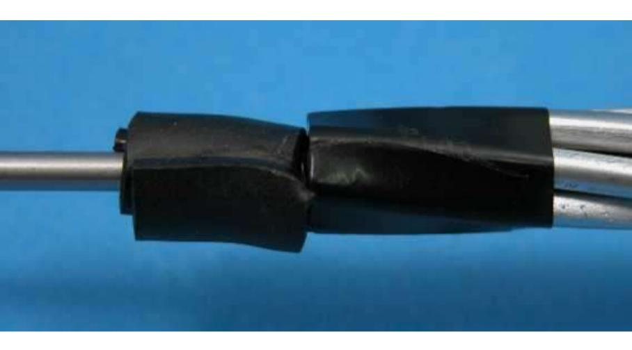
The outer layer of strands should be secured with a tie-wrap
