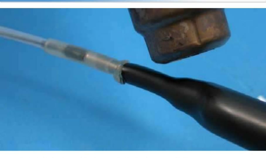
Apply the 16/5-size heat-shrink tube over the block using a controlled heat gun
