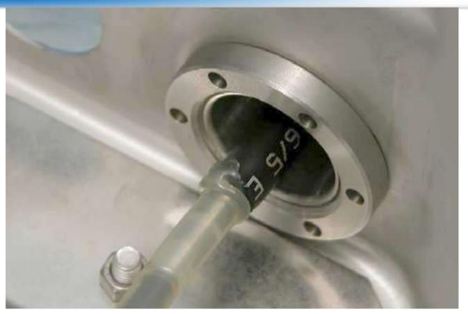
Mount the cable bushings in the outer holes using the cable bushing tool. Slide the heat shrink tube (33/8) onto the cable bushing. Put the cable thru the cable bushing until the black heat shrink tube is visible inside the closure. Apply the second heat shrink tube (33/8) with the closure cover taken of, over the cable bushing and down onto the first heat shrink tube, to complete the sealing.
