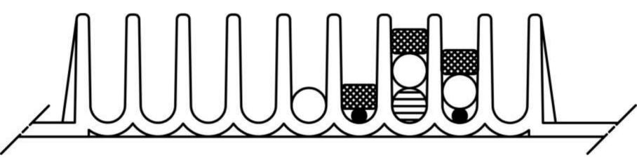
Splice the fibres and fix the splice protection sleevs in the slots with a rubber piece
