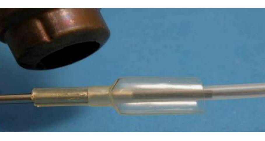
Secure the transport tube with the transparent heat-shrink tube using a controlled hot air gun
