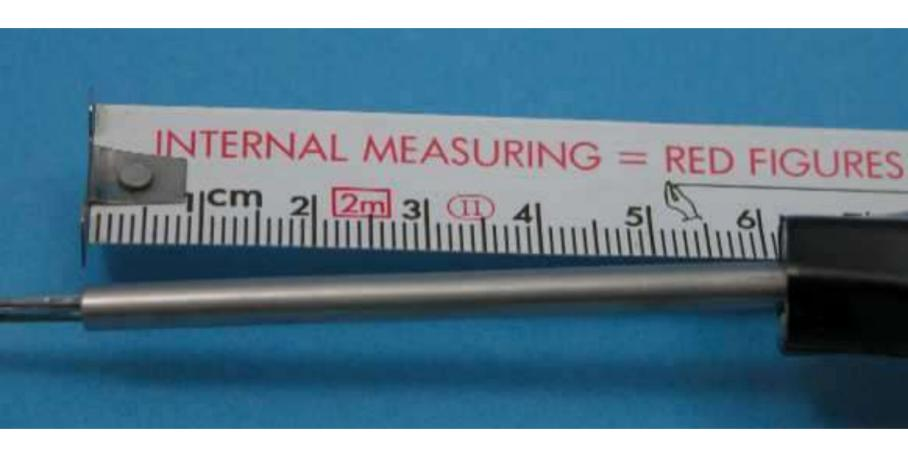
Clean and cut the fibre tube carefully 60 mm
