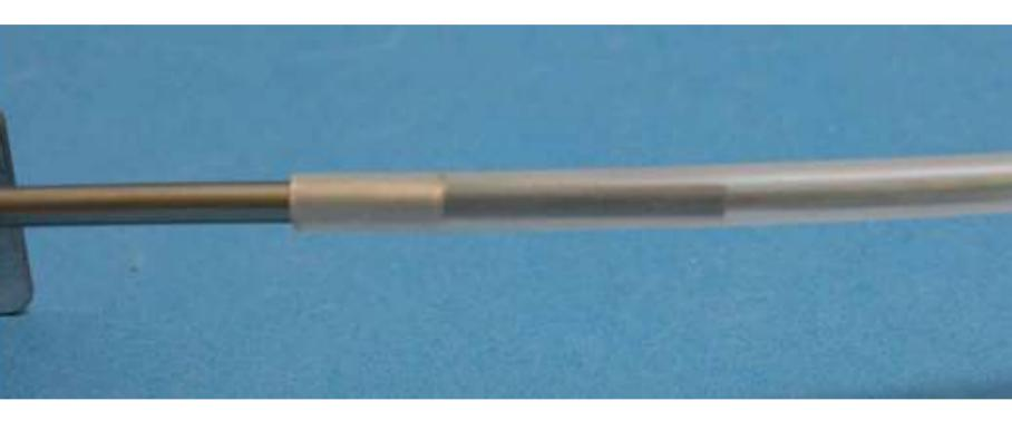
Put all fibres thru the transport tube and slide the transport tube 20 mm over the metal tube
